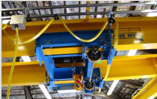
Top Running Double Girder design with custom Crab Style Low Headroom trolley.
