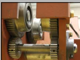
2x6 tonne Heavy Load Bearing Under Running End Trucks.
