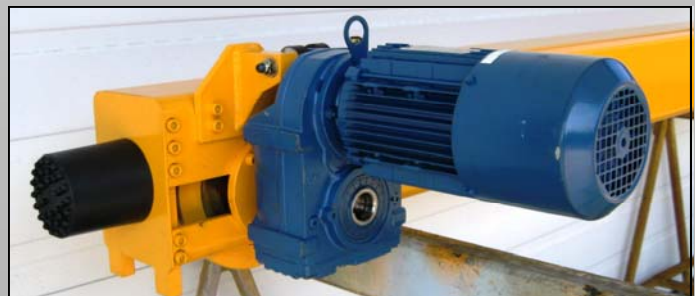
Tubular Steel End Trucks equipped with Hollow Bore Bridge Drives, Rotating Axles & Bearing Caps.
