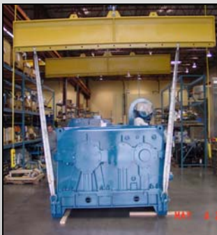
Custom Spreader Bar to facilitate the lifting of 10 magnets & controls.
