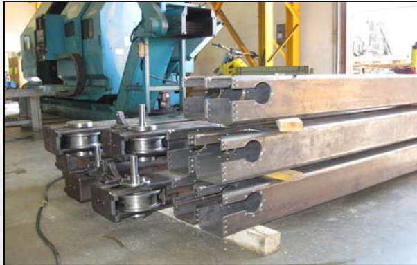
Tube Style End Trucks being machined & assembled for stock (above).
