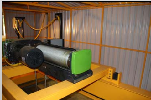
A look inside the protective housing of a Base Mounted Hoist on a Top Running Trolley (above).
