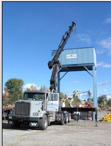
10-tonne capacity Trailer Reload Hoist structure with protective weather housing.
