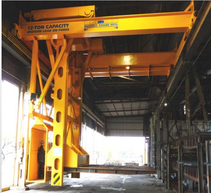
12 ton Custom Stacker Crane for a foundry.
