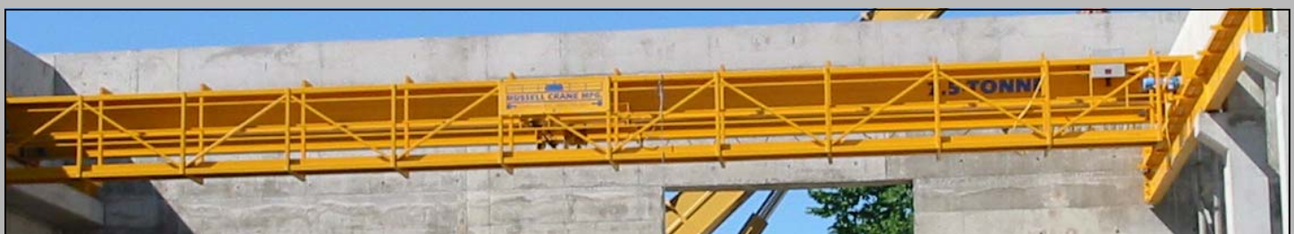
7.5 tonne Top Running Single Girder Crane with full length service platform designed for water treatment plant in Ontario, Canada (below).
