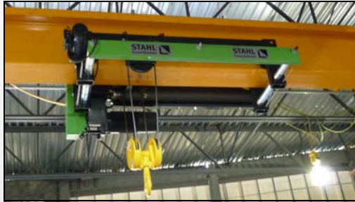
Top Running Single Girder Crane with True Vertical Lift Hoist.
