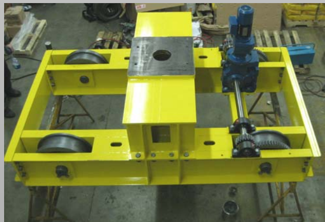
Custom Trucks for work platforms. 120,000 lb capacity per Truck.
