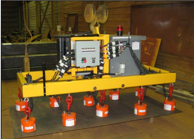
Custom Spreader Bar to facilitate the lifting of 10 magnets & controls.
