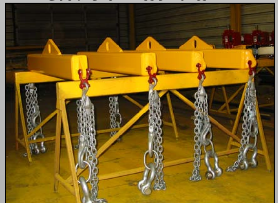
Custom Spreader Bars with Quad Chain Assemblies.
