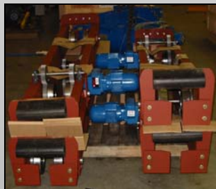
2x6 tonne Heavy Load Bearing Under Running End Trucks.
